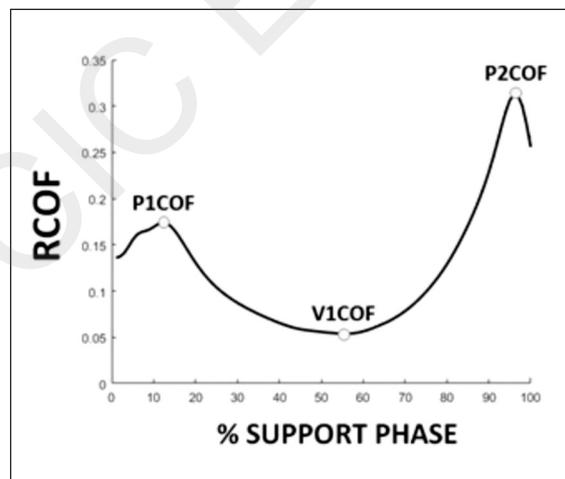
Figure 1 - Required coefficient of friction (RCOF) variables.
